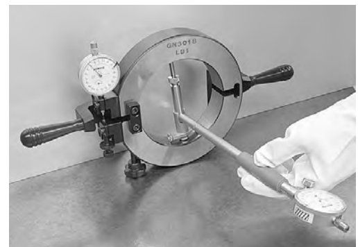
Fig. 1.9 Adjusting the GN Gauge Bore
